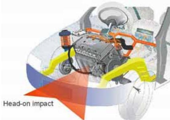
The engine will be driven back over the steering linkage. This often forces the steering wheel upwards and in higher speed impacts the airbag will deploy in line with the steering wheel. Bear in mind that in collisions between vehicles of difference masses velocity change will have the effect of increasing the Delta V force experienced by the smaller vehicle and differential in ground clearance resulting in an under-ride, will exacerbate the incidence of steering wheel upturn,
