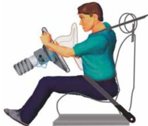
This will be further accentuated where the occupant sits too close to the steering wheel or where they are rotund and large. The airbag, as it deploys will strike the seat occupant prematurely.
