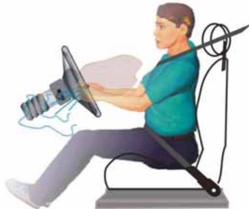
Steering wheel design was altered to house and support the airbag. The centre hub is larger and deeper and the spokes supporting the rim are shorter and more robust. The additional in-built strength coupled with airbag deployment has altered the mechanisms of injury, but before we can take this further we must appreciate how the bag deploys.
