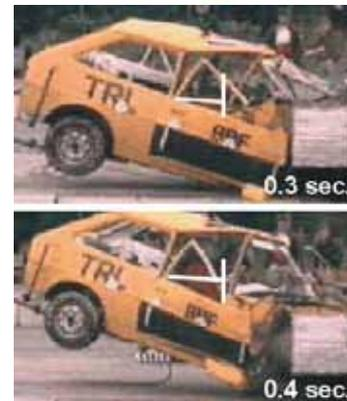
As new vehicle designs have become more substantial we see less of this, but consider, crash testing is conducted at only 40 mph (64 kph).
