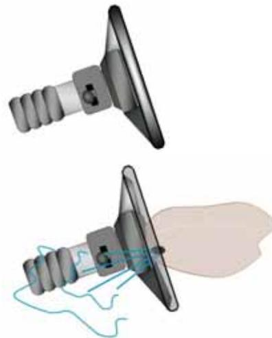
Up 2005 model year vehicles the actuating airbag will initially deploy in the shape of a tongue. The module can generate over 700 psi and deploy the bag at over 200 mph. The bag is designed to deploy as quickly as possible and in doing so it will vent excess pressure via the exhaust ports at the rear of the bag. If the bag could not vent itself it would simply self-destruct.
