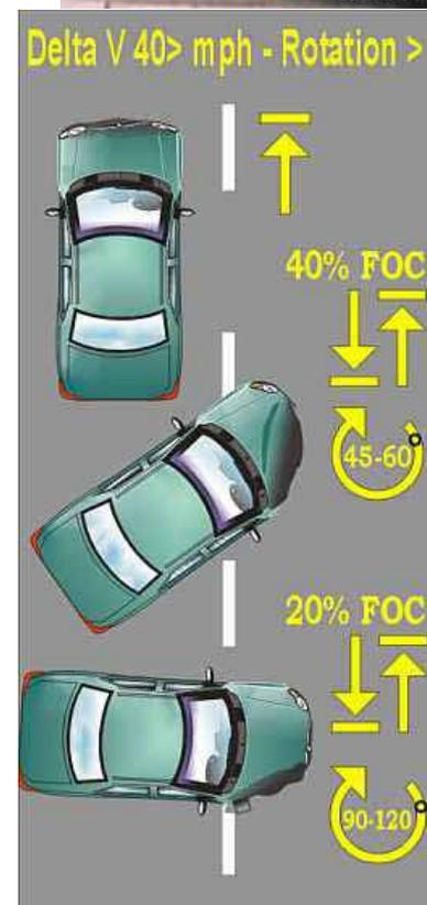
**Rebound** – The greater the speed of head-on and front 1/4 oblique impact the greater the amount of rebound can be expected. The reactionary force of metal memory retention and bounce back must be added to the Delta V force. This also adds to airbag deployment force. Therefore, rescuers should be aware of the three mechanical anomalies that can be involved –
