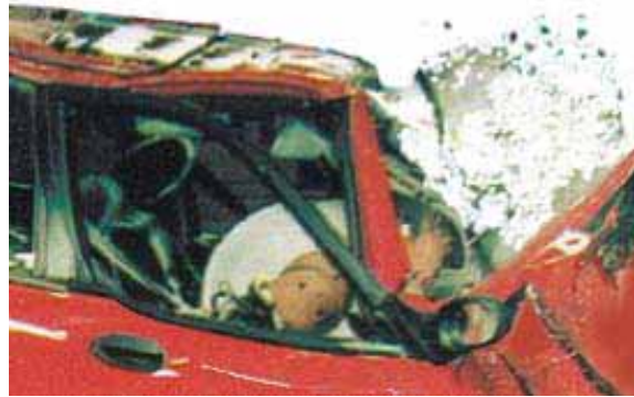
In 40% off-front crash testing the dummy's face is painted so as to measure contact with the airbag. As can be seen here the head sometimes missed the airbag and is channelled towards the intruding windscreen pillar
