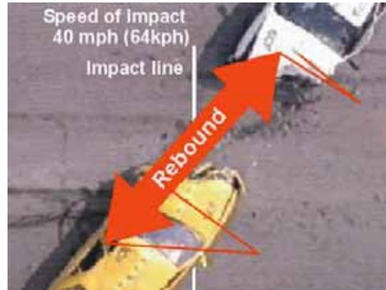
**Directional Forces** – In a collision, which is subject to high Delta V force, occupants will continue to travel in the same direction as before the impact. In the head-on impact the driver will be thrown onto the steering wheel and then projected rearward by the rebound force.
