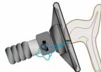
Instead of acting as a cushion, which deflates on contact, the inflating airbag will act more as a catapult, ejecting the seat occupant backwards.
