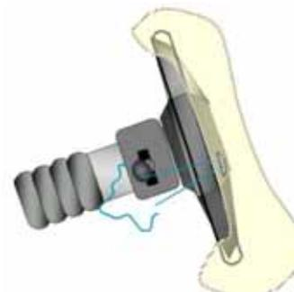
In lower speed collisions it is most unusual to see any bending to the steering wheel rim, particularly where the airbag module is housed in a large centre hub with four spokes supporting the rim. However, in the higher speed impact, the severity of injury can be indicated by the number of supporting spokes and the degree of bending in the rim.
