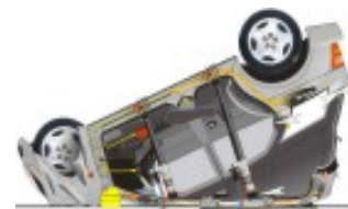
Side removal with inverted ramming and cutting
