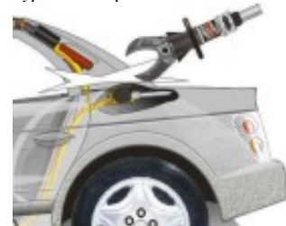
Cutting the rear roof post
