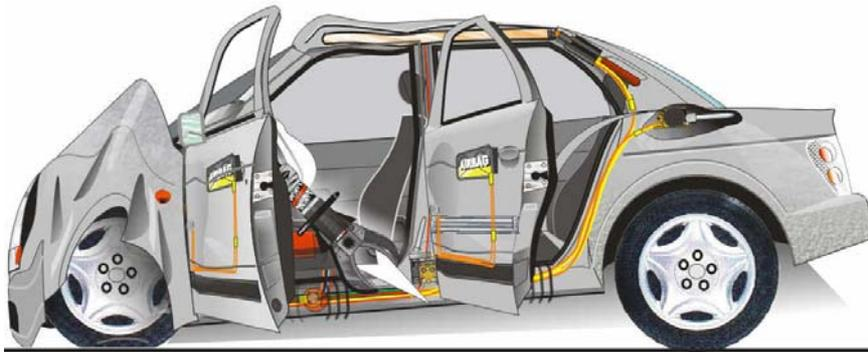
**Side Removal** - The possibility exists for short circuit or static to deploy all modules on the same system, especially where the vehicle remains energised. Inadvertent cutting can liberate Sodium Azide/Sodium nitrate – For more information go to [www.resqmed.com/SRSlogicBm.pdf](http://www.resqmed.com/SRSlogicBm.pdf)
