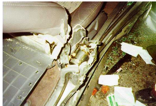
'Side removal' performed using a combi tool carries the highest risk of inadvertently cutting through the pretensioner module.
