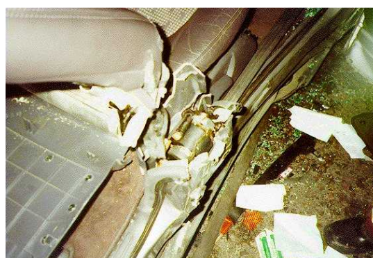
'Side removal' performed using a combi tool carries the highest risk of inadvertently cutting through the pretensioner module.
