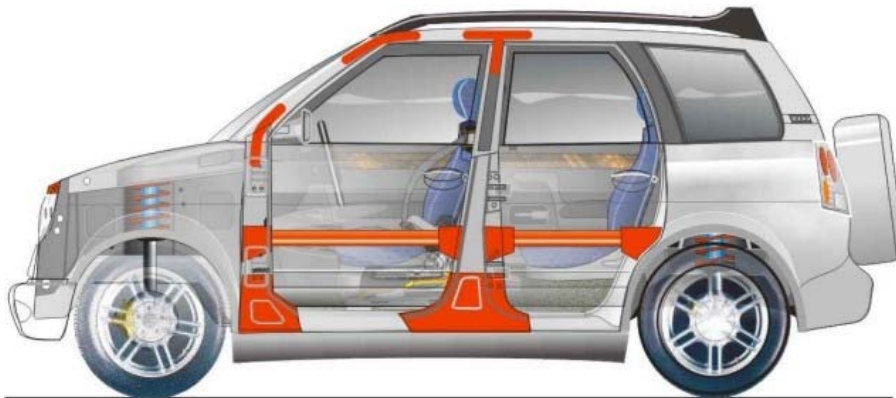
Strengthening bars, gussets and plates
