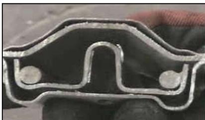
Many rescue tool manufacturers’ display their cutters shearing through strengthening bars and HSLA channel with Boron steel bar inserts. Be aware of the cross sectional area in respect of the cut. Where the channel is small it will butt up against the stock where the tool has the most cutting force. This display of the cutters ability is not a true indication of what is actually required.
