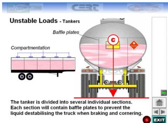
The tanker is compartmentised into a series of separate tanks. Again baffle plates are constructed within each tank to minimise movement of fluid during transportation, especially when cornering and braking.
