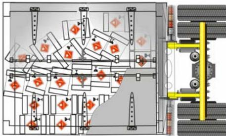
Where the truck/trailer has come to rest on its side, movement in the cargo is virtually guaranteed. The coachwork structure will be either prefabricated or framed. Either way it will have little substance and the cargo will have to be unloaded before a lift can be entertained. Hazardous material, leakage or spills must be guarded against and special precautions taken where necessary.
