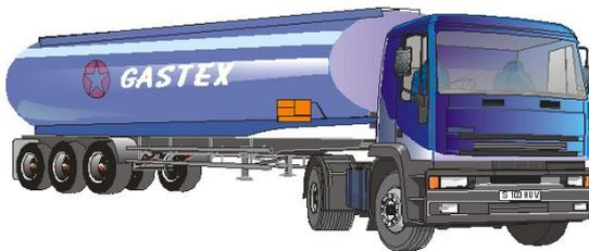
Tankers present problems all their own. The tank is divided up and can have up to five or more compartments. Each compartment will be sub-divided with interconnecting baffle plates to mitigate the movement of fluid when braking and cornering. However these plates only prevent the sudden rush of fluid; they do not prevent the eventual settling and levelling of the fluid. Where the tanker is parked on a camber or incline, the fluid in each compartment will adjust to that level relatively quickly.
