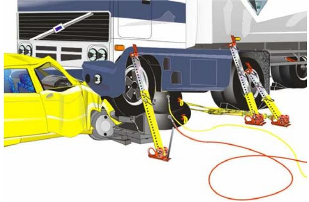
**Cribbing, packing or purpose made chocks.** Blocks and wedges are essential, not just for supporting the lift, but also in preventing lateral movement. Some chocks offer good support while others are next to useless. It is necessary to use interlocking blocks 'up side down' to use the wedges to best advantage. I still put my trust in good old-fashioned stress graded wood.
