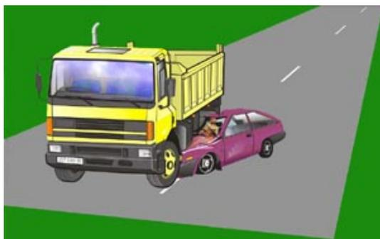
*Many trucks are equipped with less than adequate under-ride side bars and some have none at all. With some side-on under-rides it may be necessary to separate the car from under the truck. This becomes more complicated where the tandem rear wheel rides up onto the car crushing the bulkhead and forcing the steering wheel, column and dash onto the driver.*
