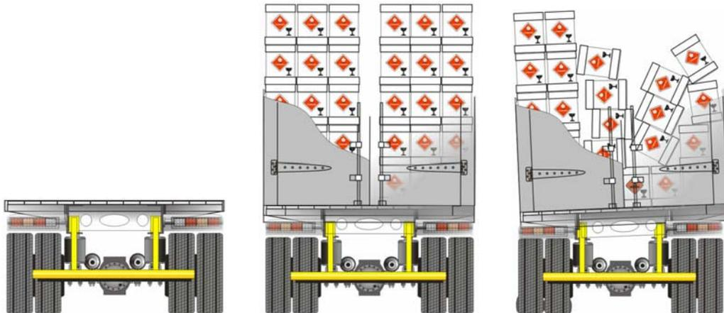
How a truck's cargo is distributed and secured is very important to the centre of gravity of the vehicle. Even where an unladen truck or trailer is positioned on a gradient of 2% or more the centre of gravity alters accordingly and any lifting must take this into account. On some occasions this can
