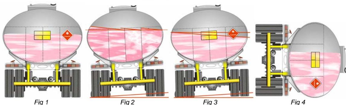
Initially the fluid will overflow the baffle plates (Fig 2) and quickly find its level (Fig 3). As the fluid overcomes the restriction and inertia it will alter the C of G. Unless this has been taken into account for it can lead to uncontrolled movement and, with some situations, has been known to topple the load.
